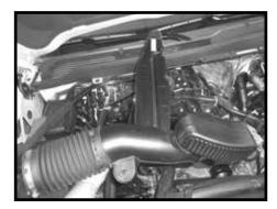
Step 5 Remove the factory air intake tube and resonator assembly from the vehicle.
